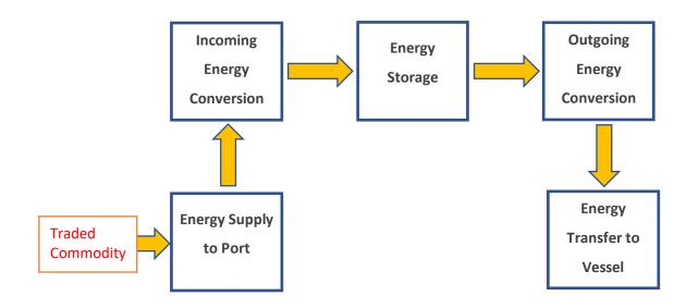
Energy processing and conversion systems needed in each module are defined, depending on the energy vector being used to bring the energy resources into the port (the 'Traded Commodity') for which a market price is available. The complete system is then modelled to determine the overall system efficiency, the cost (of buying energy and of financing the capital investment) and the net carbon impact.
